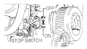
Figure 6. Engine On/Off Switch
